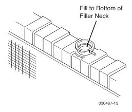
Figure 7-10. Coolant Level
